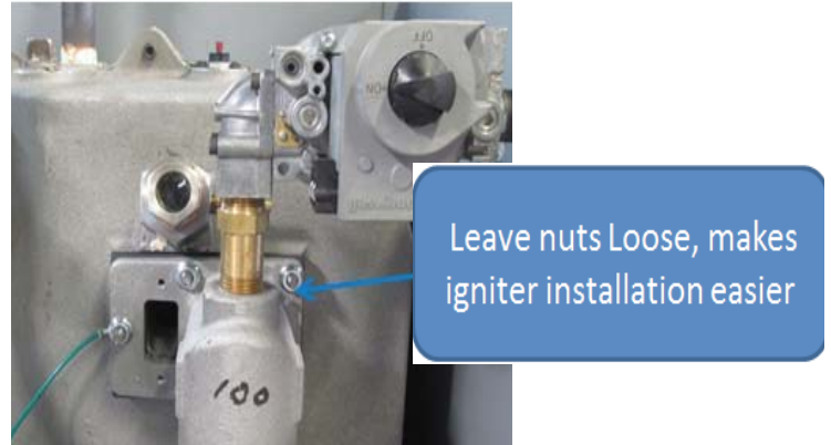
Figure 17 Install Hot Surface Igniter
