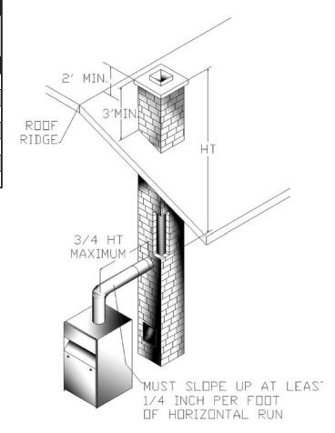
Accessibility clearances must take precedence over fire protection clearances. 18" clearance should be maintained at a side where passage is required to access another side for cleaning or servicing, inspection, or replacement of any parts that normally may require such attention. 18" clearance is recommended on the control side for servicing.
