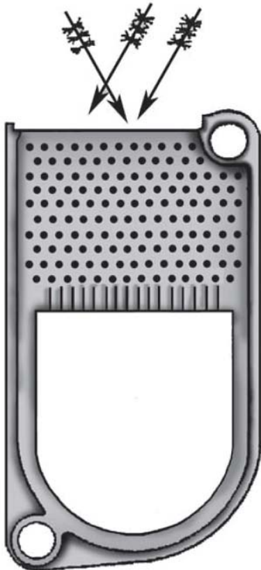
Figure 14 - Brush Diagonally Through Flue Passages
