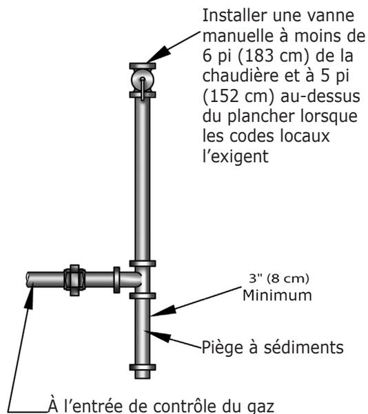
**FIGURE 7-2 Emplacement de l'orifice de gaz**
