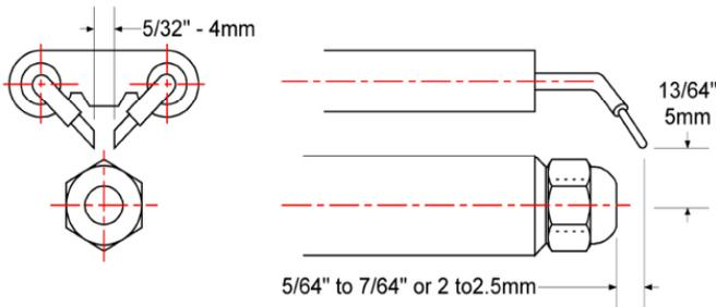
Figure 17 - Riello Turbulator Setting
