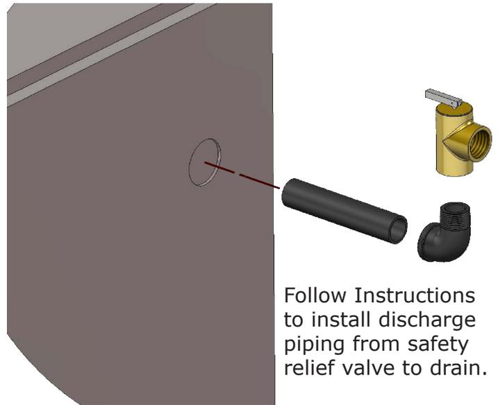
Figure 6b - Discharge Piping From Safety Relief Valve
