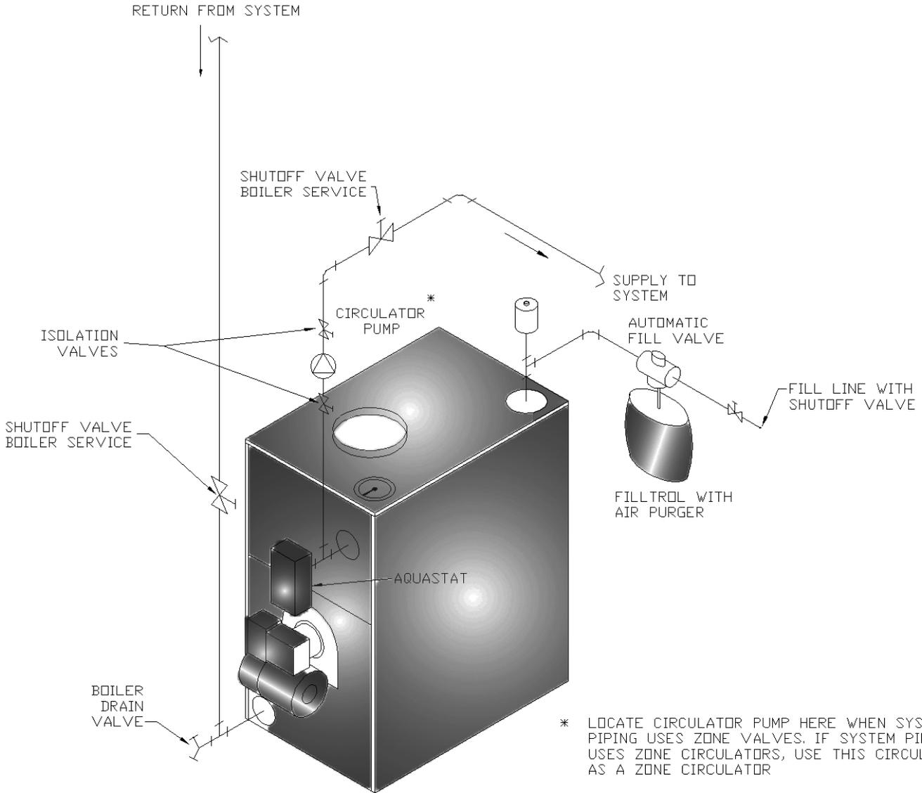
Tankless Coil Piping Arrangement
