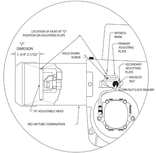
Figure 16 - Riello Electrode Setting
