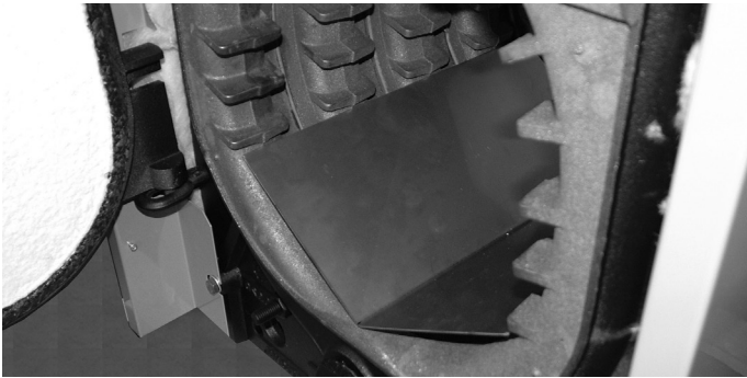
Figure 12 - V-Shaped Liner
