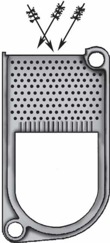
Figure 19 - Brush Diagonally Through Flue Passages
