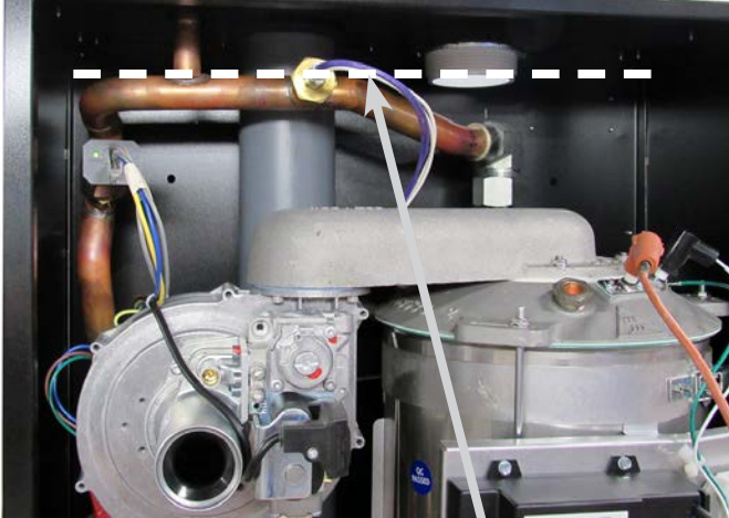
Figure 5 - Manual Reset LWCO Minimum Acceptable Height (200 Size Boiler Shown)
