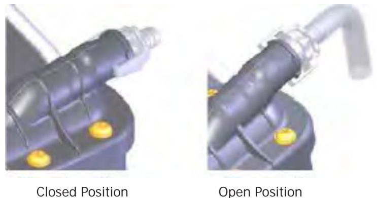
FIGURE 9-5 Manual Deaeration Valve - Top Of Heat Exchanger
