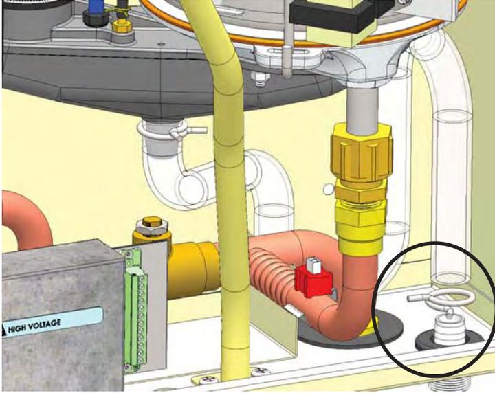
1. Disconnect collet clip from hose barb and fill Condensate trap with water.
