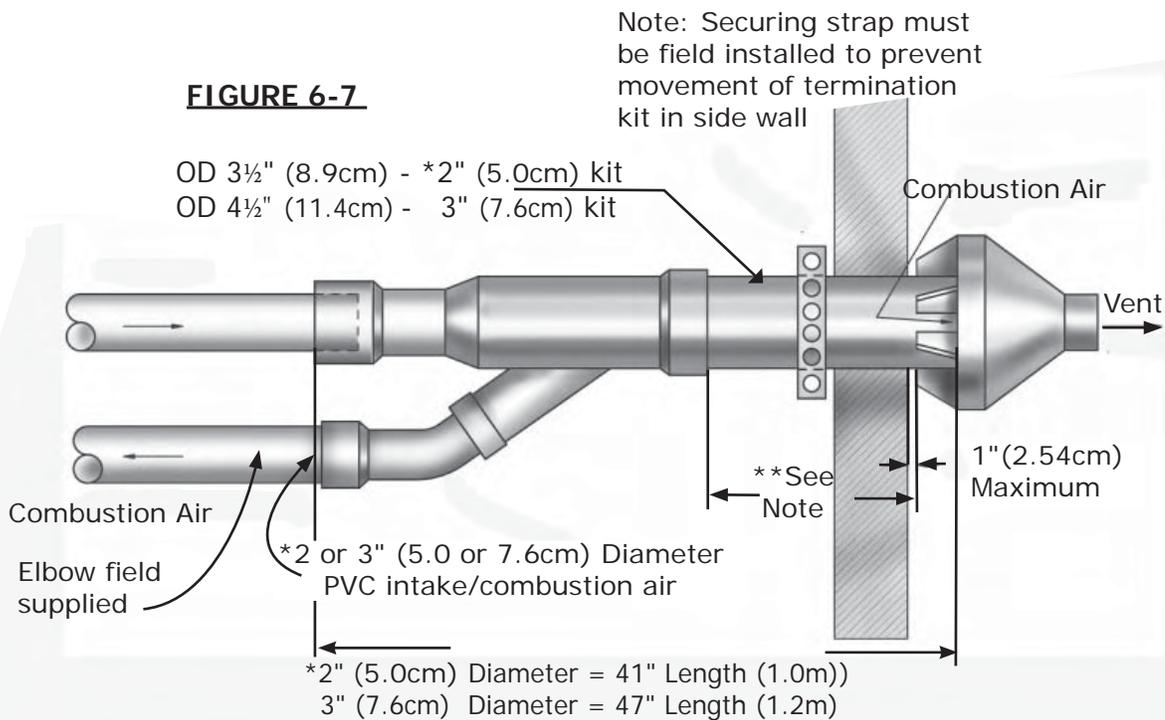
\*\* Note Overall length may be modified by cutting or extending both combustion air and vent pipes. 12" is minimum allowable length and 60" is maximum allowable length for this dimension. SDR-26 PVC (D2241) only may be used for extending pipes. Do not use Schedule 40 PVC or use couplings to extend pipes. Dimension will change if intake/vent pipes are lengthened or shortened.
