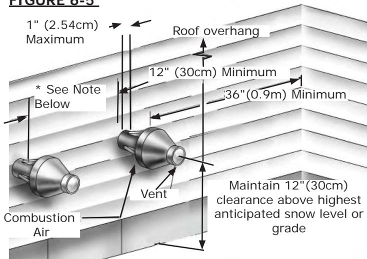
\*Must be less than 4" or greater than 24" Horizontal distance between end bells of each air intake to prevent flue gas recirculation.
