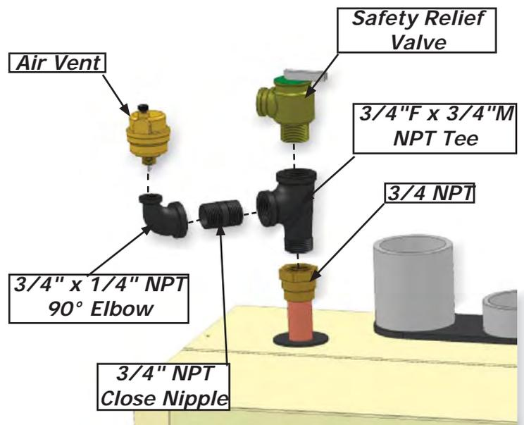
Position Air Vent and Safety Relief Valve to provide space for discharge piping.
