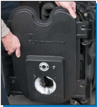
Reversible hinged door easily lifts off hinges and positions right or left
